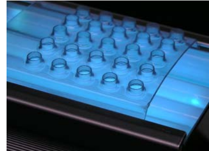
The optional Light Brush™ helps clear hair so UV light can get to the scalp.
